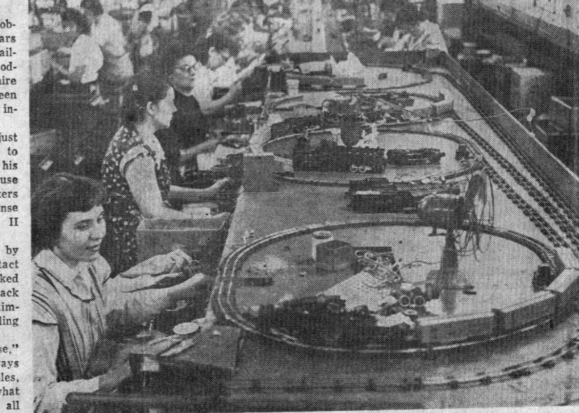
PART of Gilbert's test line. It costs as much to bring out a new 'toy' loco as it does to build a real one, now that precision is all-important.
