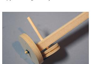
**Step 3.** At the other end of the arm, put a large wheel on the peg sticking out the end of the arm (put the o ring on the outside to hold it on) and put the smaller wheel with the dowel in it up through the hole next to the large wheel.
