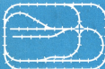
No. 10—Space 80" x 120" Track Required 30 Curve 42 Straight 1-1/2 Straight 3 pr. of Switches 1 Crossover
